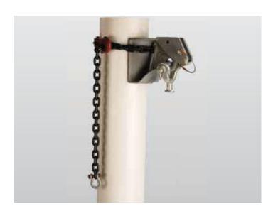
The S+R Model GK-200 "armless" pole bracket is made to accommodate two Model XS-100-B Universal blocks. One block can be mounted either in the vertical position or on an angle using the side lug. The second Universal block is suspended below and is free to assume any line angle. Ideal for poles with "armless" design, the GK-200 is adjustable to fit different diameter poles: wood, steel, aluminum, or concrete, without drilling or marking them.
