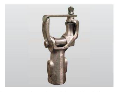
Equipped with two polished all aluminum alloy rollers to support the conductor during straight stringing and angles up to 10°, the PM-1-AG has a clamp top to keep the wire (or pulling line) from coming out where an uplift exists. This limited-use block fits down onto standard NEMA pins 1"-1 3/8" and with adapter will screw directly onto standard 1" NEMA pin.
